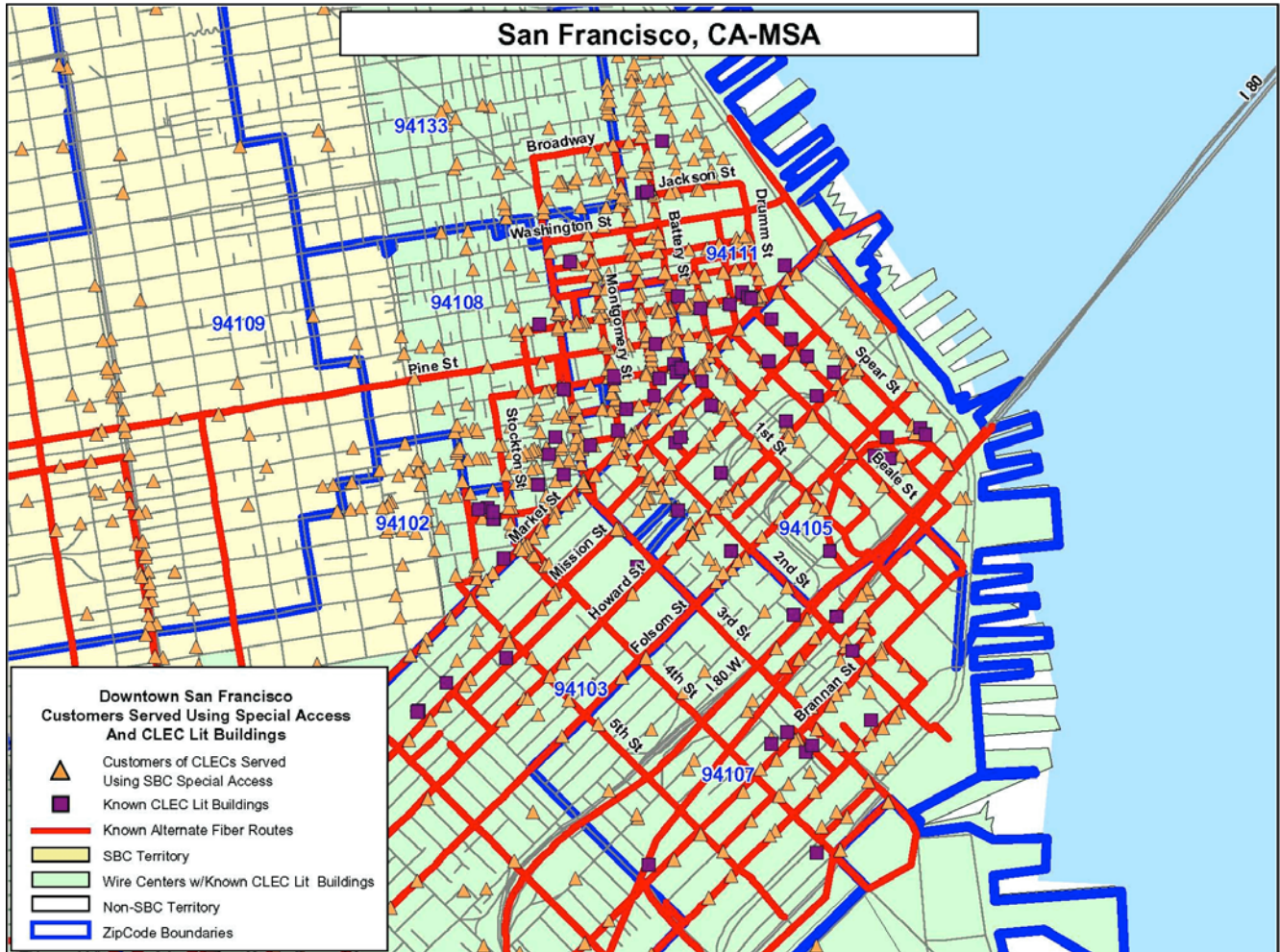
Figure 1. Competitive fibre optic cable deployment and use in the San Francisco financial district showing CLEC enterprise customers being served using Special Access even where CLEC fibre routes are adjacent to the customer’s building.
