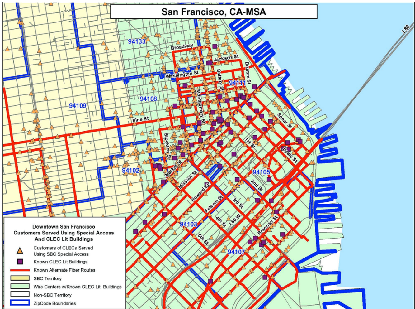
Figure 4. Competitive fibre optic cable deployment and use in the San Francisco financial district showing CLEC enterprise customers being served using Special Access even where CLEC fibre routes are adjacent to the customer's building.
