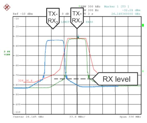
of time when 'green' is attempting to receive a distant signal near the noise floor, it appears as interference.
