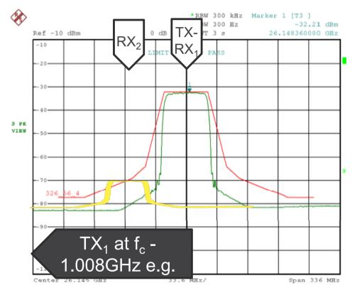
The FDD receiver suffers interference from the TDD transmitter.
