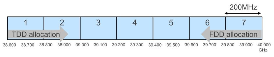
Note — this effectively creates dynamically-sized TDD and FDD sub-bands, restoring the status quo of homogeneously duplexed contiguous spectrum.
