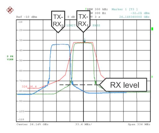
incompatible systems. Even if it is possible, it wastes capacity and prevents arbitrary TX-RX scheduling. Usually a fixed ratio and master network are chosen (e.g.LTE-TDD).
