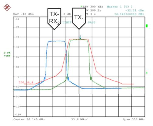
The TDD receiver suffers interference from the FDD transmitter.
