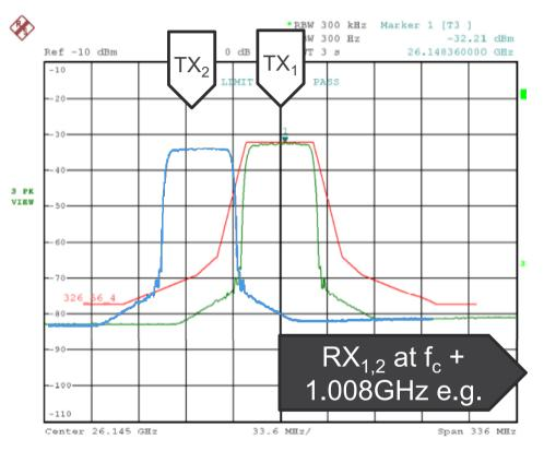
carrier frequencies are sufficiently distant in frequency that there is no remaining leakage from the adjacent co-located transmit channel.
