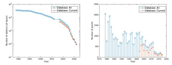
**Figure 1.** The number of earth stations of different types has significantly decreased since the 1980s (left). Similarly, the number of new grants is also falling (right), showing overall that the mid-band 3.7-4.2 GHz is likely underutilized currently.<sup>6</sup>
